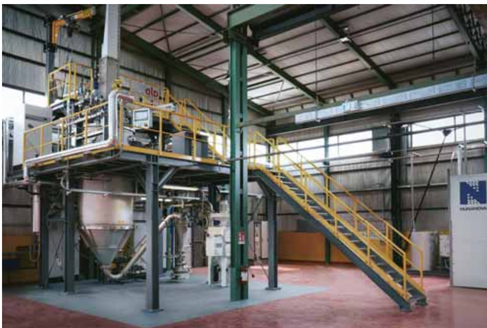
Impianto EIGA - Electrod Induction Gas Atomisation
